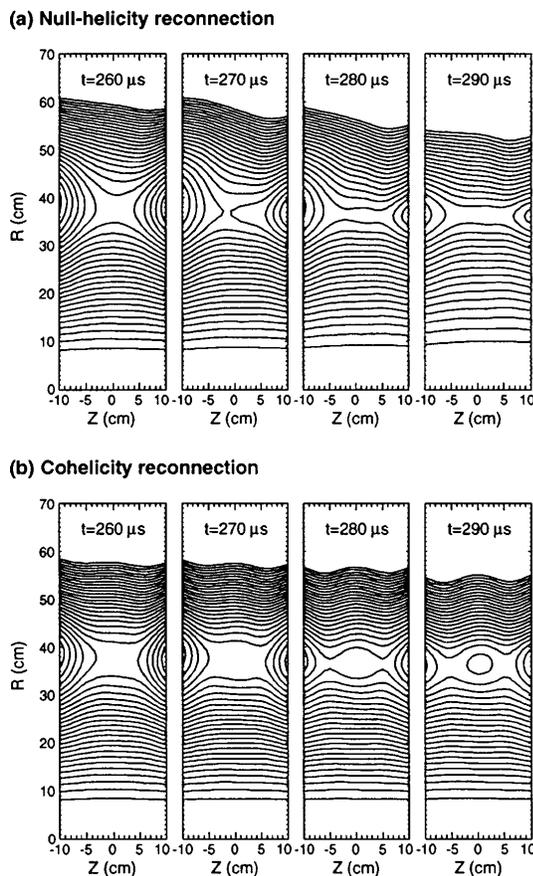
FIG. 3. Time evolution of  $\Psi$  contours (in 0.5 mWeb intervals) measured by internal magnetic probes in 6 mTorr  $\text{H}_2$  discharges. TF and PF capacitor bank voltages are 10 and 8 kV, respectively. The equilibrium field is 150 G at the center of the machine. Double-Y-shaped and O-shaped diffusion regions are formed in the (a) null-helicity case and (b) cohesivity case, respectively.
