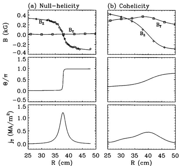
FIG. 5. Radial profiles of measured  $B_Z$ ,  $B_T$ , field line angle ( $\Theta$ ), and  $j_T$  at  $Z = 0$  cm and  $t = 290 \mu\text{s}$  in the (a) null-helicity and (b) cohesivity cases (TF and PF bank voltages are 12 and 10 kV, respectively, and the EF field is 200 G).
